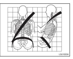
The lap part of the belt should be worn low and snug on the hips, just touching the thighs. In a crash this applies force to the strong pelvic bones so you'd be less likely to slide under the lap belt. If you slid under it, the belt would apply force at your abdomen. This could cause serious or even fatal injuries. The shoulder belt should go over the shoulder and across the chest. These parts of the body are best able to take belt-restraining forces.
